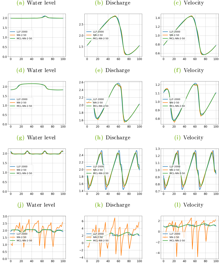
Figure 6.6: SWE with initial conditions illustrated in Fig. 6.2. Discretizations at T = 40 were obtained with Heun's method on periodic meshes.
