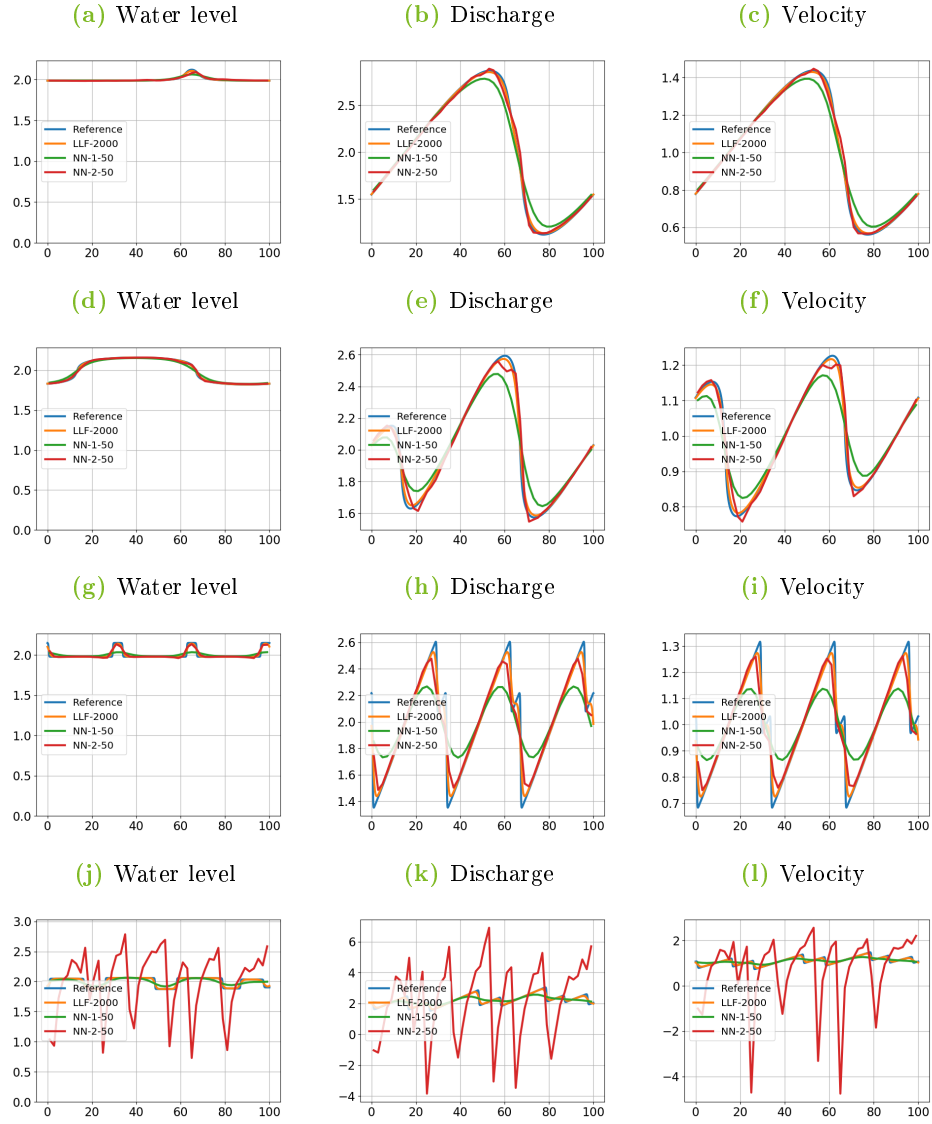
Figure 6.4: SWE with initial conditions illustrated in Fig. 6.2. Discretizations at T = 40 were obtained with Heun's method on periodic meshes. The reference discretization is generated with an LLF scheme on a uniform mesh consisting of 10000 cells.
